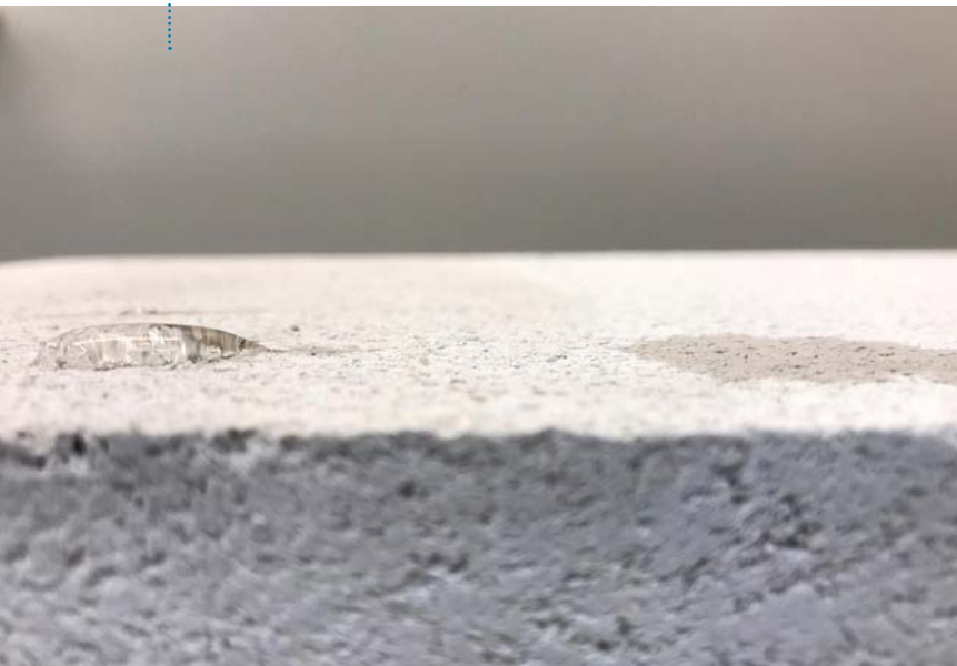
Fig. 2 & 3: AAC functionalized with CEMsil SC-I on the left and no treatment on the right with water on top
