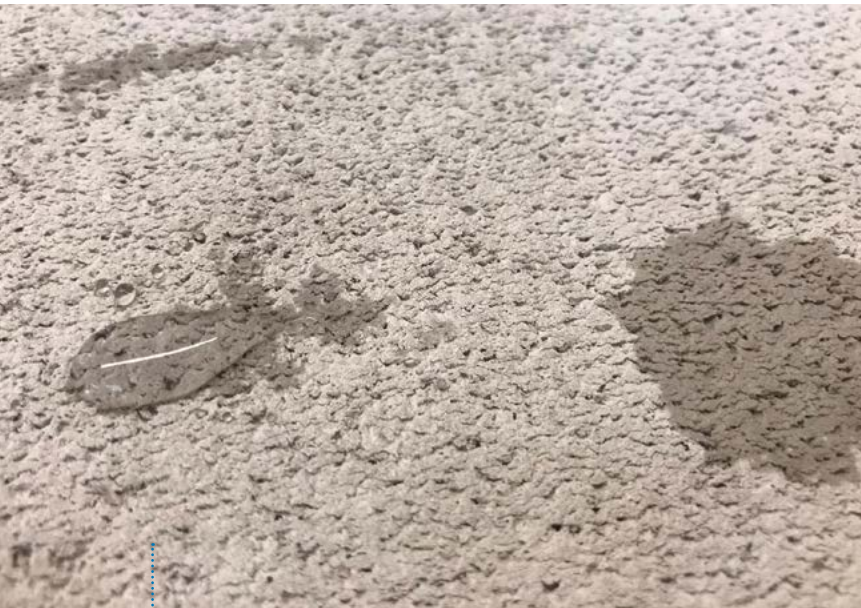
Fig. 2 & 3: AAC functionalized with CEMsil SC-I on the left and no treatment on the right with water on top
